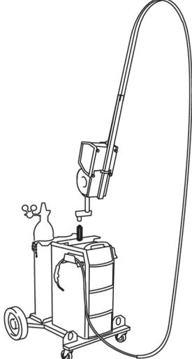
A line drawing of Trolley 2, which is similar to the first trolley but includes a counterbalance device. The counterbalance device is a long, curved arm that extends upwards and then back down to the trolley. It is attached to the feeder. |
