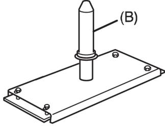
A line drawing of a guide pin. It consists of a vertical pin with a conical tip, mounted on a rectangular base plate. The base plate has four mounting holes. A label (B) points to the insulating bushing on the pin.                        |
